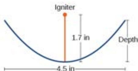
**Figure 13** Cross-section of a travel-sized solar fire starter
